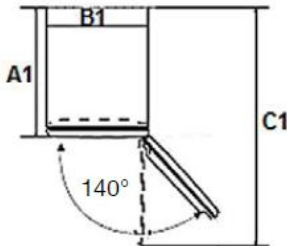
**A 1= Depth / B 1 = Width / C 1 = Depth (when the doors are open) / D 1 = Space requirement of the appliance (width) when the doors are open / door opening angle 140°**
